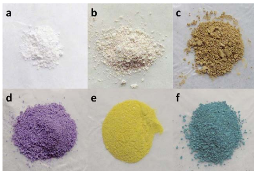
Figure 3. The colors of different \text{Na}_3\text{MPO}_4\text{CO}_3 carbonophosphates: M = Mg (a), Mn (b), Fe (c), Co (d), Ni (e), and Cu (f).
